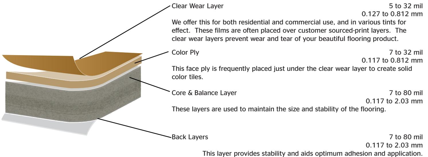
Properties listed do not constitute a warranty or specification. Test values are based on material conditioned and tested in a controlled laboratory using established standards and procedures. Properties vary based on embossed grain, color, multi-ply lamination and other variables.
