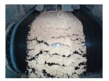
The ContiClean® A-H conveyor belt does its job successfully because of its purpose-designed anti-stick coating. In practice the new development has turned out to be ideal for conveying sticky materials such as:
