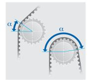
The larger the arc of contact, the more teeth mesh with the pulley and the greater the loads that can be transmitted. In the case of multi V-belts, the contact surface area with the belt pulley increases analogously.
