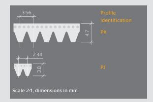
Elastic multi V-belts can be labeled with two lengths: 1. The production length and
