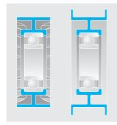
Idlers with flanges are termed guide pulleys. They keep the timing belt on the required track. If a flanged tensioning pulley is used, no additional guide pulley is required. Left: Idler
