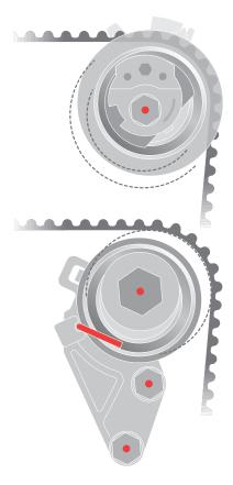
The tensioning systems' pivots and attachment points are marked in red.
