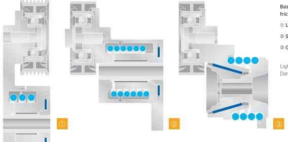
Basic forms of mechanical, friction-damped tensioners:
