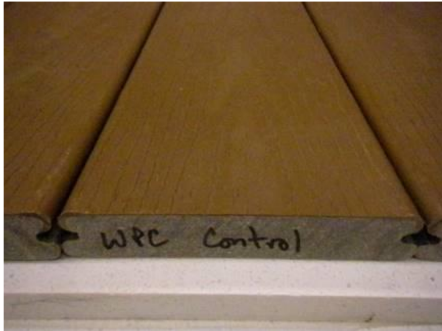
Photo No. 5 Specimen #5 Identification - WPC Control Deckboard
