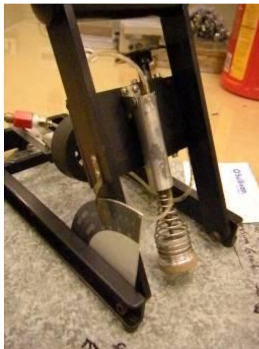
Photo No. 6 VIT Slip Resistance Test Equipment
