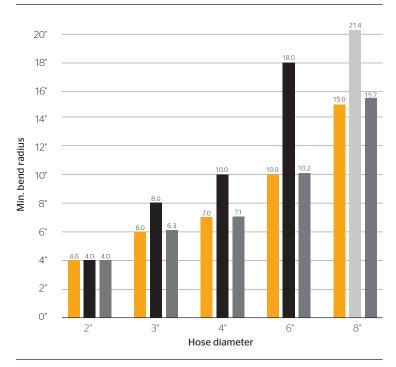
Minimum bend radius is a measure of resistance to kinking. Velocity hose outperformed the competition in nearly every size - especially the larger diameters.
