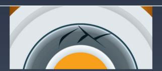
Damage due to extremely high use of idling position, e.g. a taxi.
