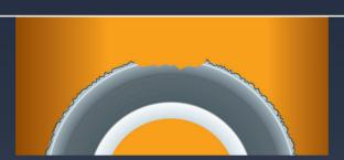
Overheating on the outer ring as a result of belt slippage.
