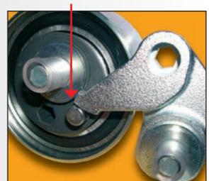
Lever correctly positioned
