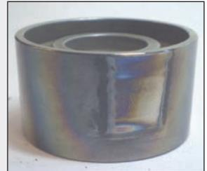
Idler pulley mechanically seized (engine side up)
