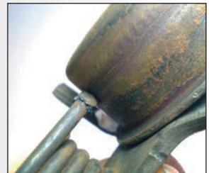
Contact between spring and running surface
