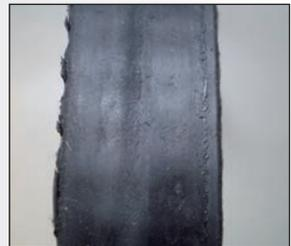
Overheated back of the timing belt
