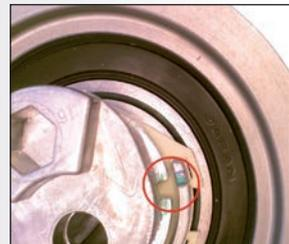
Tensioning pulley mark
