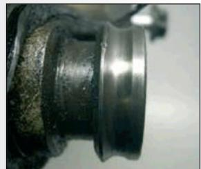
Journal of the tensioning pulley retaining plate
