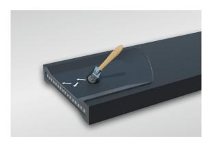
) Using a hand roller and working from the center outwards, press the patch firmly into place, making sure that no air pockets form.
