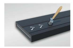
Press firmly into place with the help of a hand roller, making sure that no air pockets are formed. If air bubbles occur, they can be removed with a needle by puncturing the bubbles.
