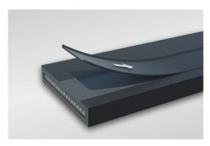
) Place CONREMA repair material in damaged area.
