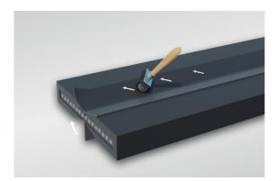
Thread first ply of coated repair material through the tear, wrapping it around the top and bottom sides of the cover.
