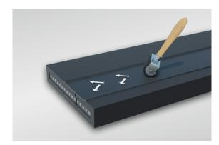
) Roll down firmly with hand roller, working outwards from center to avoid formation of air pockets.
