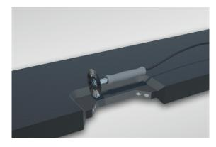
) Using a rotating wire brush, to rough up the enlarged cut-out area thoroughly. (Working ca. 10 mm beyond the area traced).
