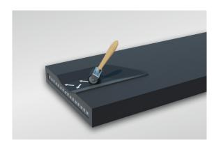
) Using hand roller, press firmly into place, rolling outwards from center. Make sure no air pockets are created.
