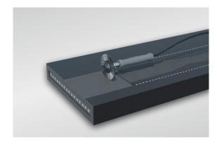
Remove patch and rough up the area carefully, working 10 mm beyond traced-out area in all directions.
