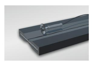
Thoroughly rough up cut-out areas on both sides of cover with rotating wire brush (sanding roughly 10 mm beyond the damaged area).
