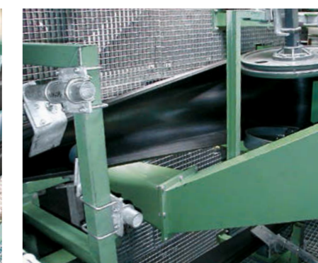
Does not pollute thanks to enclosed belt on return trip
