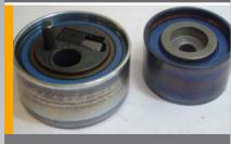
The belt components become overheated after a short period of running (pulley seizure). AII: 3.0 DTI V6
