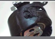
The tensioning roller shows pronounced indications of melting on the lagging. AII: 1.2-16V
