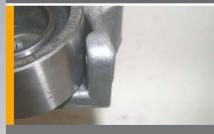
The tensioning pulley becomes misaligned under the load on the bracket and seizes. AII: 2.0 / 2.5 V6
