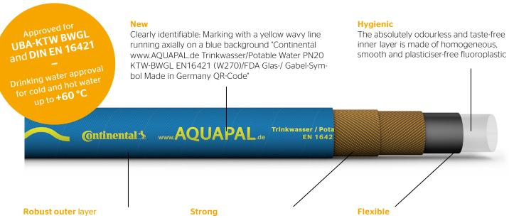
NBR, blue, fabric-patterned, abrasionresistant, oil and grease-resistant, ozone, weather and UV-resistant Synthetic yarns make the AQUAPAL® resistant even to high pressures (operating pressure 20 bar/290 psi)
